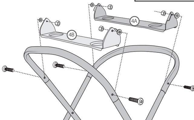
Using the wider bath support (4A) for the wider set legs and the narrower bath support (4B) for the narrower set legs, place the bolts through the leg tubing so that just enough bolt is poking through to slide the washers onto the bolts (see fig1). Place the bath supports between the legs and then, push the bolts all the way through.
