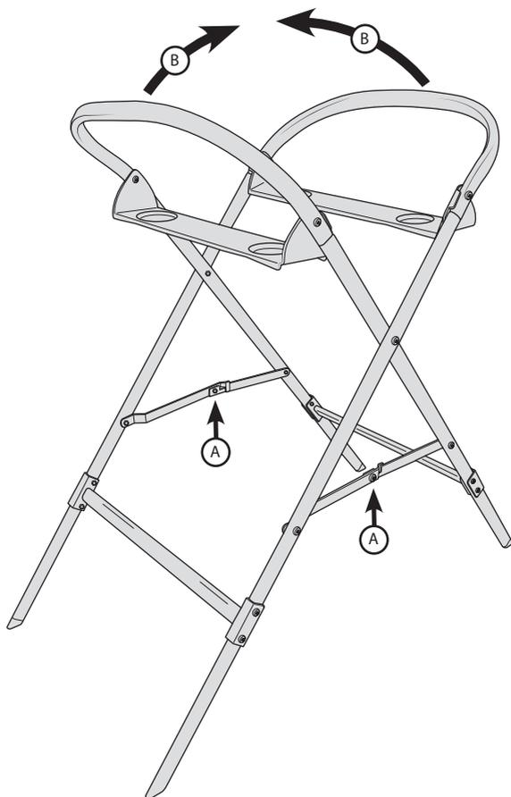
To fold: Unlock both braces (A) by raising them in the centre by approximately an inch. Holding the two top rails, draw them together (B).
