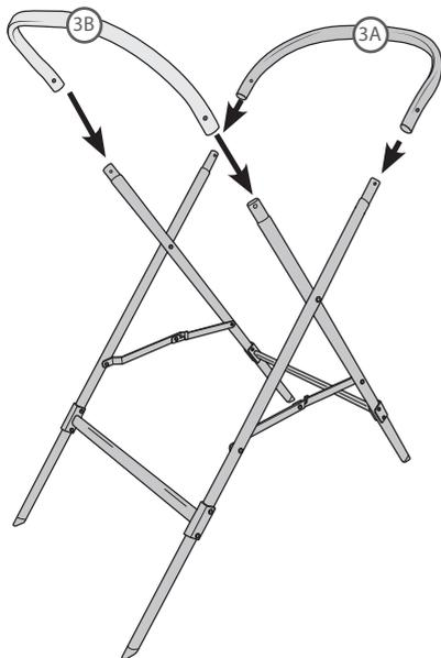
Using the wider top rail (3A) for the wider set legs and the narrower top rail (3B) for the narrower set legs, push the open ends of the top rails onto the ends of the legs.
