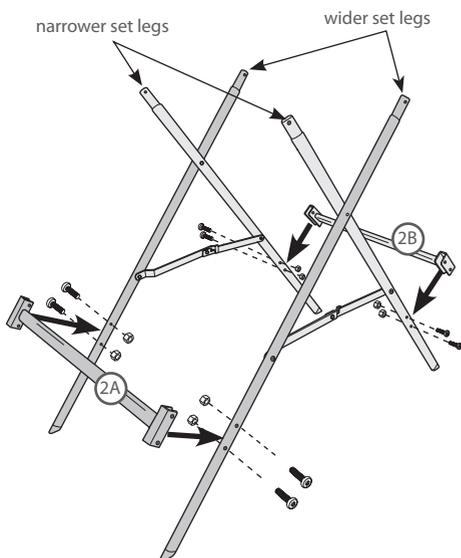
Using the wider strut (2A) for the wider set legs and the narrower strut (2B) for the narrower set legs, join the two sets of legs and secure using eight bolts and eight nuts.
